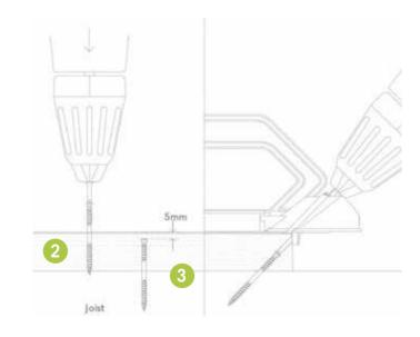
For best results, coat the fixings in silicone spray before use. When screwing in, push firmly on the screw whilst applying pressure to the board (2), finishing the screw head 5mm below the Lastane® surface. This should leave a minimal witness mark (3).
