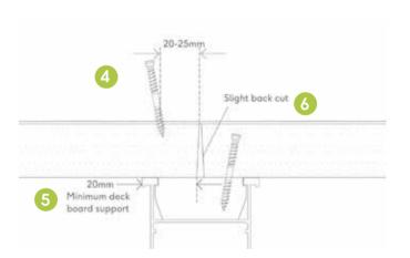
Then fix to the remaining joists. We recommend checking the boards against the string line every 4-5th row. As there may be slight variation in width, length and thickness, packers can be used to create a flat finish between two boards. Therefore it is best for screws to be left at butt joints until both boards are together.
